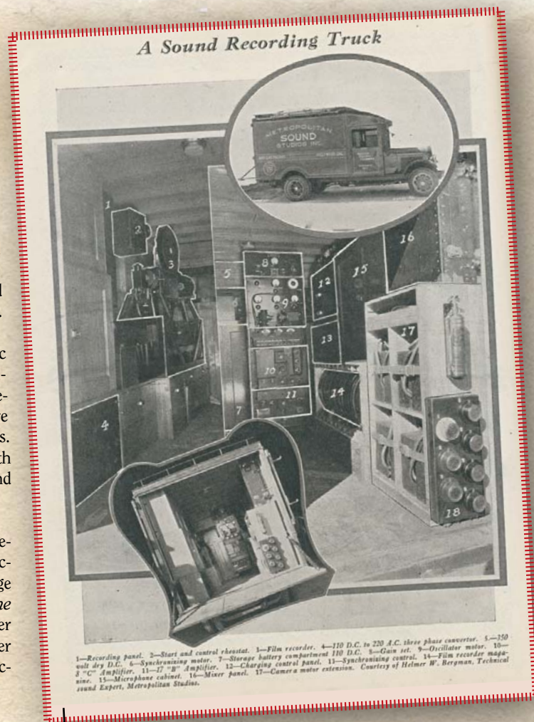
Metropolitan Studios sound truck ca. 1929. This truck, equipped with a Western Electric optical sound recording system, was typical of those in use at many studios in the early 1930s. Note the fire extinguisher at the rear—a handy thing to have when working with nitrate base film. No wireless mikes here!! (Photo courtesy of International Photographer)
