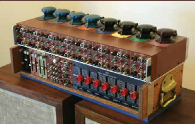
Custom mixer with modified Altec Program and Graphic EQs built with Paul Bennett.
