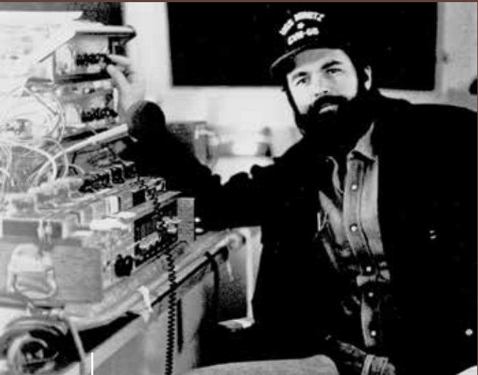
On the USS Nimitz, starboard side of the bridge. Note the double Nagra rig and the David Ronne-inspired outboard microphone preamps on top of the modified Altec equalizer.
