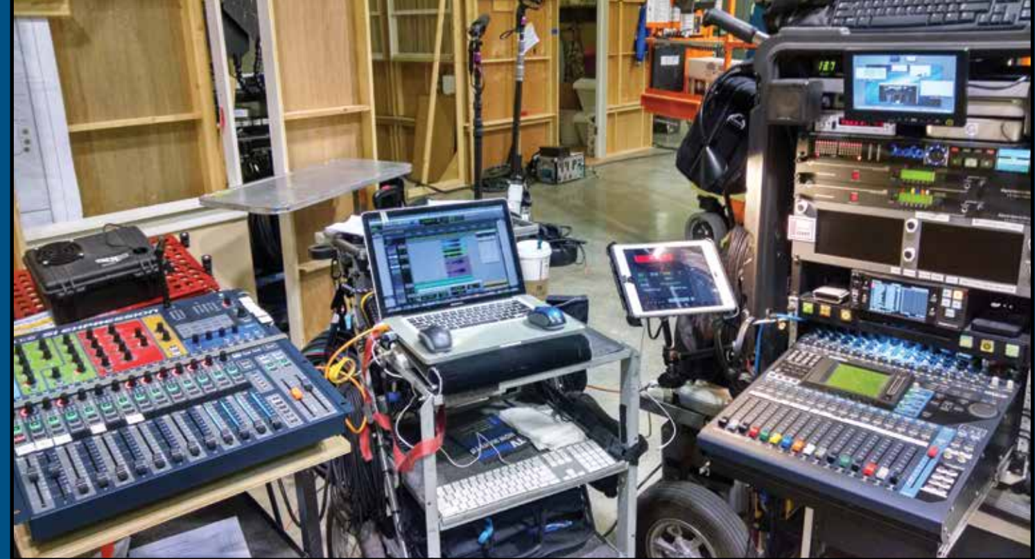
Richard Lightstone's Dante setup; Soundcraft Expression 1, MacBook Pro running Pro Tools, Main Mix cart, networked with CAT-6e cable
