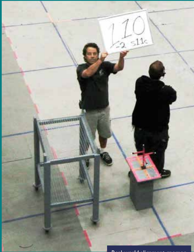
Real-world alignment gnomon and "transparent" table with wire-mesh surfaces. (Photo: 'AVATAR' ©2009 Twentieth Century Fox. All rights reserved)
