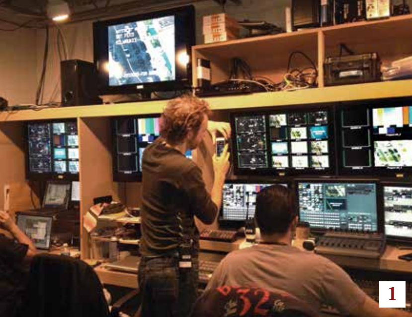
1. In the control room, the video crew used the GlobeCaster switcher to combine live and pre-built elements. The “on-air” video was then routed out to the GNN studio monitors.
