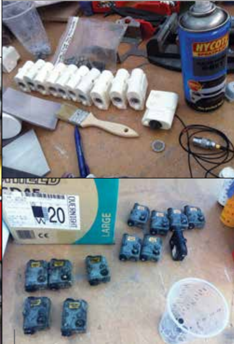
Rugged boxes were drilled to hold the microphones and painted to match the armor.
