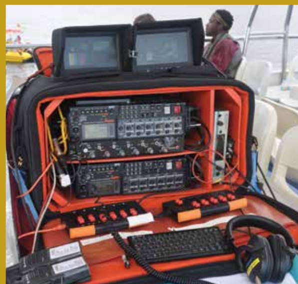
Chris Munro's "at sea" rig with two linked Fostex PD606 recorders for up to 16 tracks.
