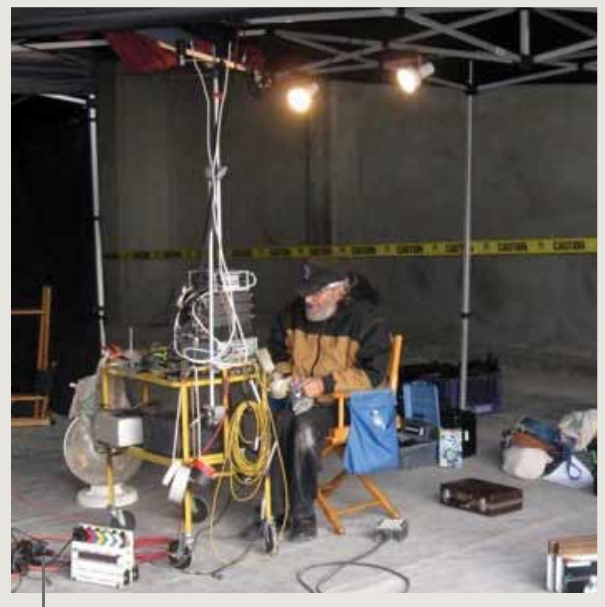
My lightweight rig—running on batteries. Four sharkfins feed a 4-pac and 6-pac of Zaxcom receivers connected to a Fusion-12. A fifth feeds my video monitor. The only two cables send an audio mix to the Codex recorders and receive playback audio from a video display image appearing in the shot.
