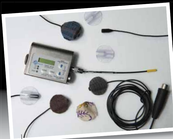
Lectrosonics SMV, DPA 4071 lavalier microphones with DPA 'concealer' mounts and costume fabric swatches to assist disguising the microphones.
