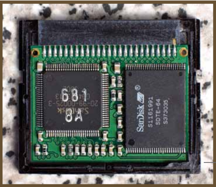
The interior circuits of a CF card. The controller is on the left and the memory chip on the right.
