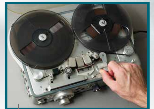
Squeezing the Nagra pinch roller—the original "Hold the Roll"
