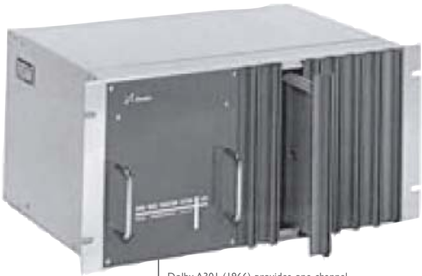
Dolby A301 (1966) provides one channel of Dolby “A” noise reduction
