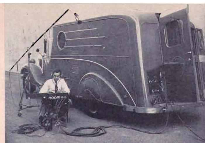
6—Modern film recording truck, built in 1936. Fred Arndt is shown at the mixing panel.
