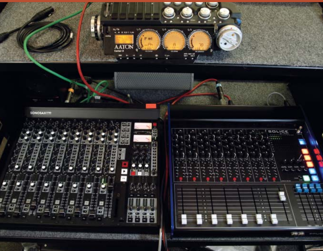
Solice vs. Sonosax SX-ST. Panels were tested side by side with an Aaton Cantar used for A-B monitoring and level calibration
