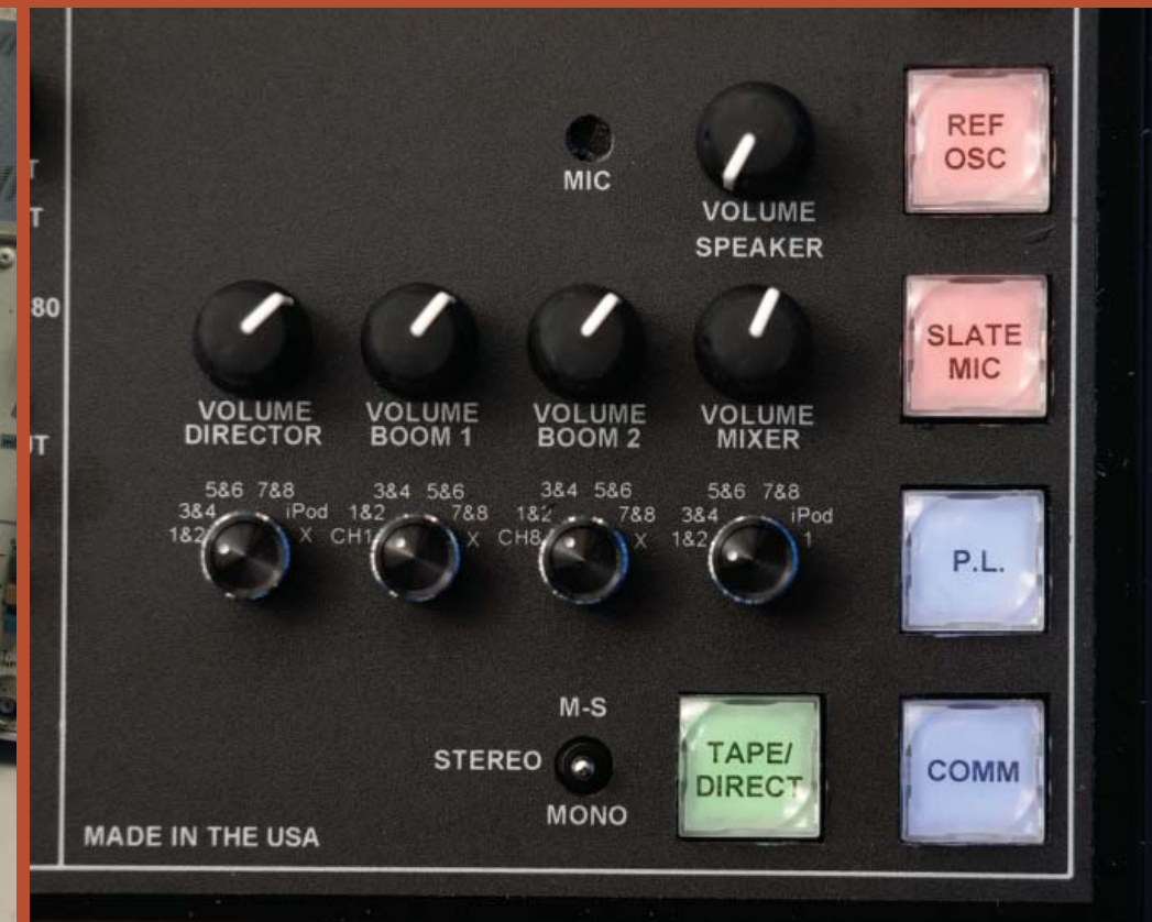
Each of the four headphone outputs has an independent routing switch and volume control
