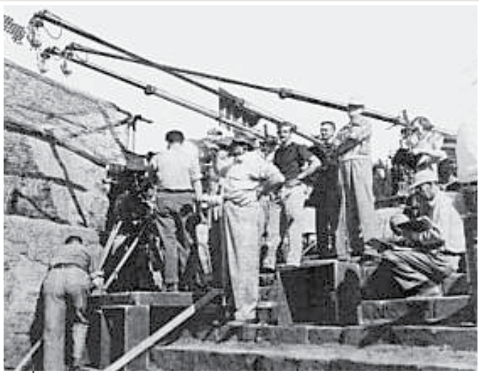
Production photo for The Robe , showing implementation of three mike booms for stereo production tracks.
