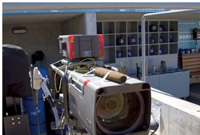
Microphone mounted on field-level camera
