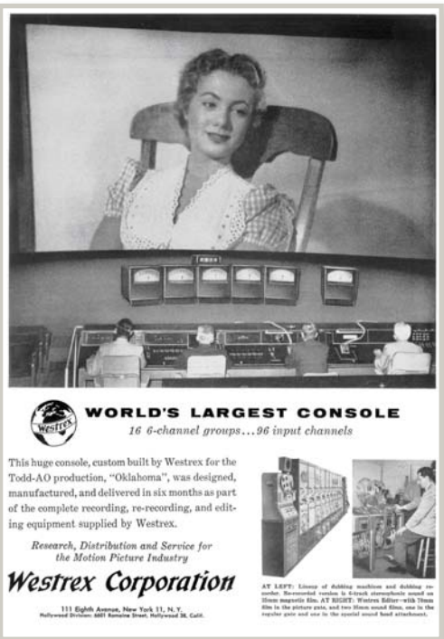
Ad showing the Westrex console commissioned by Todd-AO for the mixing of Oklahoma! 96 inputs was probably a record in those days!
