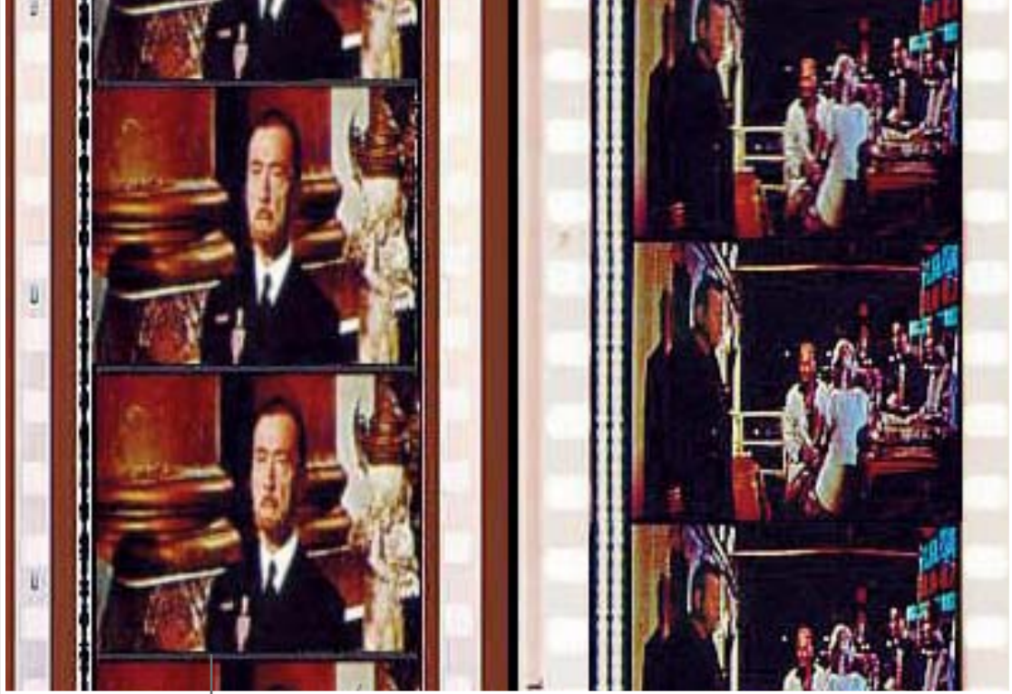
Comparison of 35mm CinemaScope four-track “Magoptical” print (on left), as compared to standard CinemaScope mono optical track. Notice that the optical track on the “Magoptical” print is half the width of a standard 100 mil mono track.
